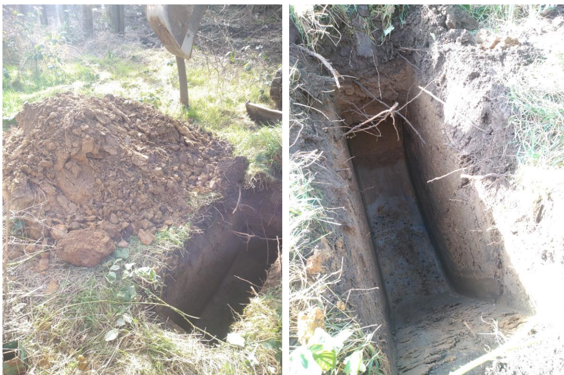
Plate 9: Photo showing location and side walls of TP2.
